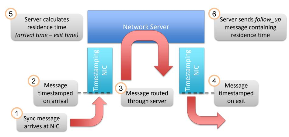
Enables deployment of full timing support on standard servers using timestamping NICSs
