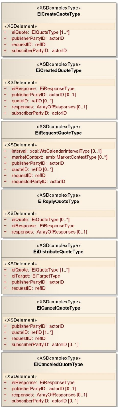
1579 1580 Figure 7-7: UML Class Diagram for the EiQuote Service Operation Payloads
