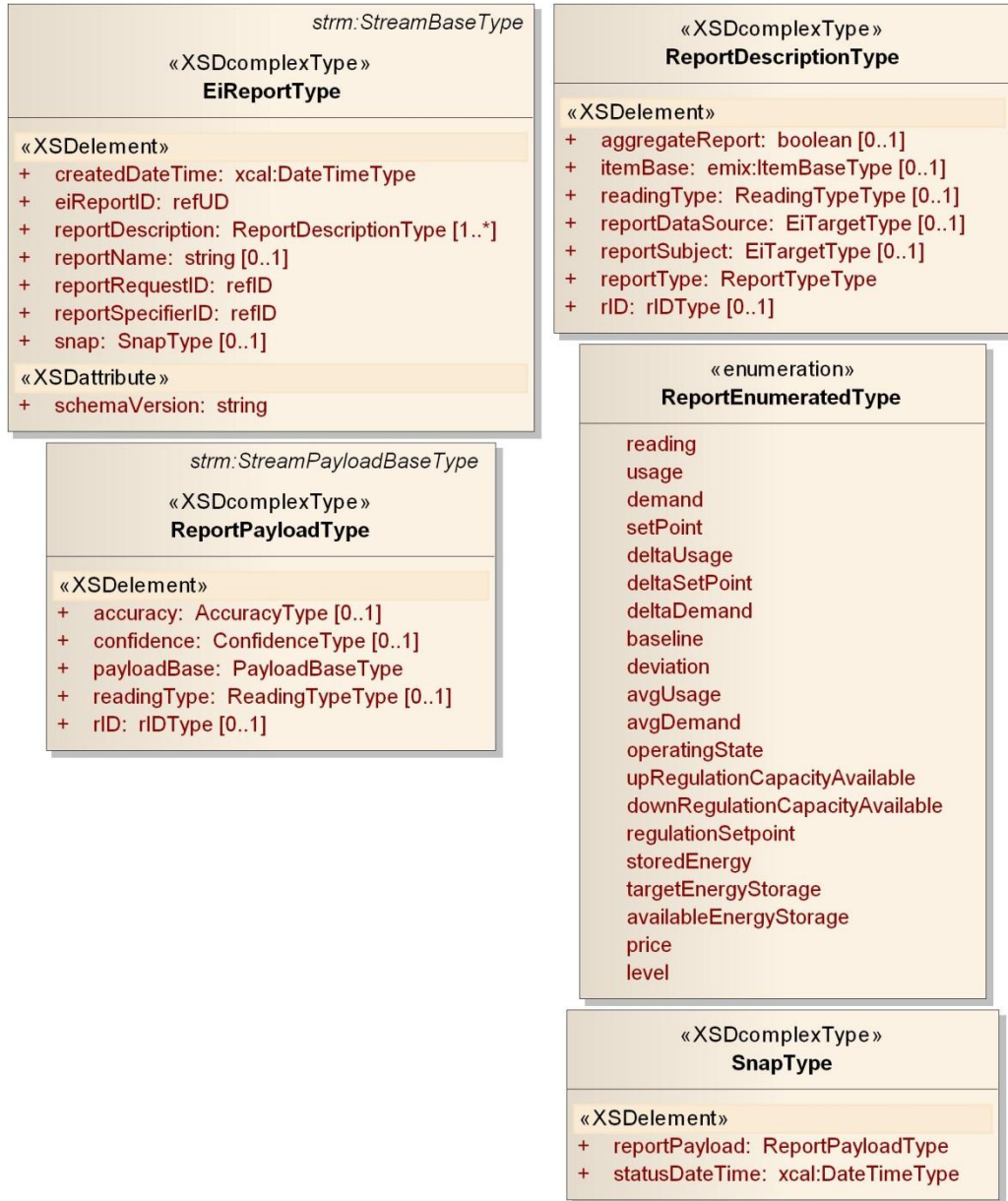
Figure 5-16: UML Class Diagram of Reports
