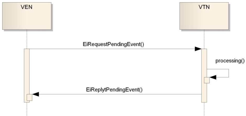
Figure 9-7: Interaction Diagram for Pending Event operation
