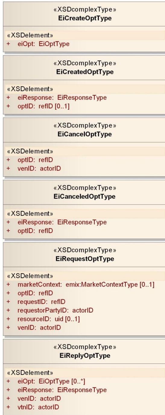
Figure 11-6: UML Class Diagram for EiOpt Service Operation Payloads
