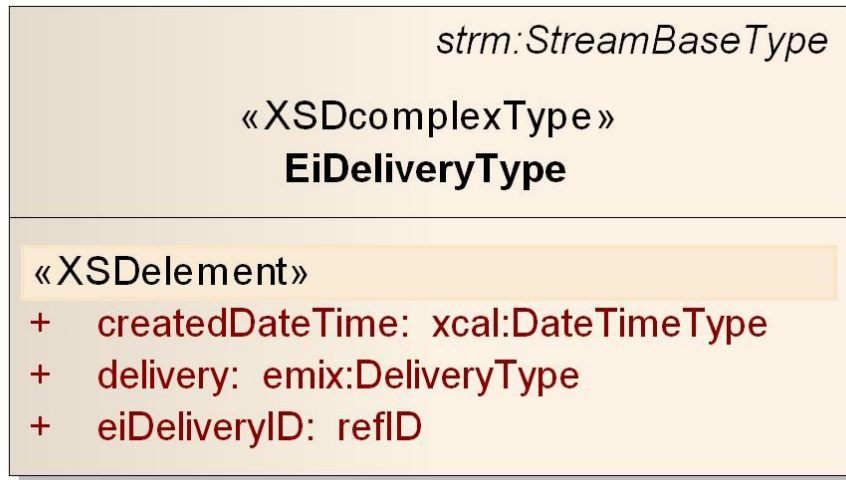
Figure 7-12: UML of EiDelivery Type
