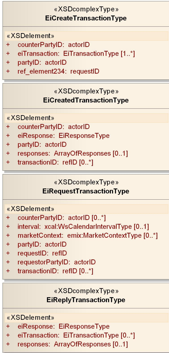
Figure 7-9: UML Class Diagram of EiTransaction Service Operation Payloads
