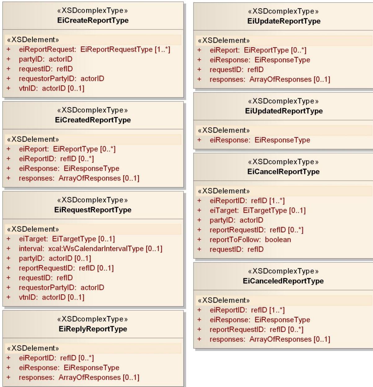
Figure 10-4: UML Diagram of Report Payloads
