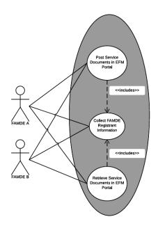
Figure 1: Central registration service facilitates Limited eSOP message exchanges on behalf of FAMDE subscribers. The EFM portal could optionally host service documents to guard against errors that can occur when document(s) exchanged exceed email gateway file size limitations.
