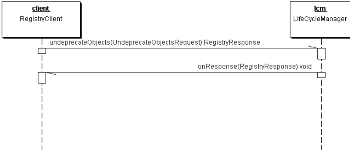
Figure 27: Undeprecate Objects Sequence Diagram
