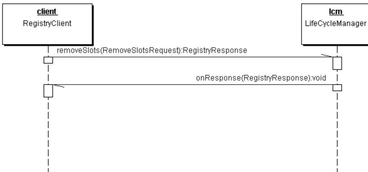
Figure 21: Remove Slots Sequence Diagram
