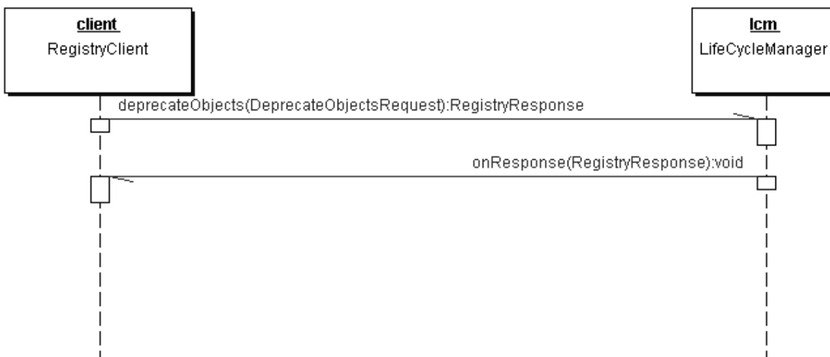
Figure 25: Deprecate Objects Sequence Diagram
