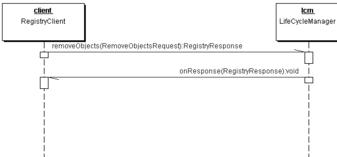
Figure 29: Remove Objects Sequence Diagram
