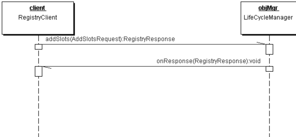
Figure 19: Add Slots Sequence Diagram
