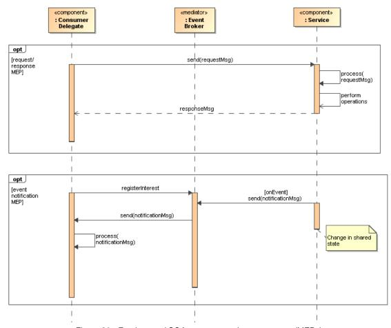
Figure 30 - Fundamental SOA message exchange patterns (MEPs)
