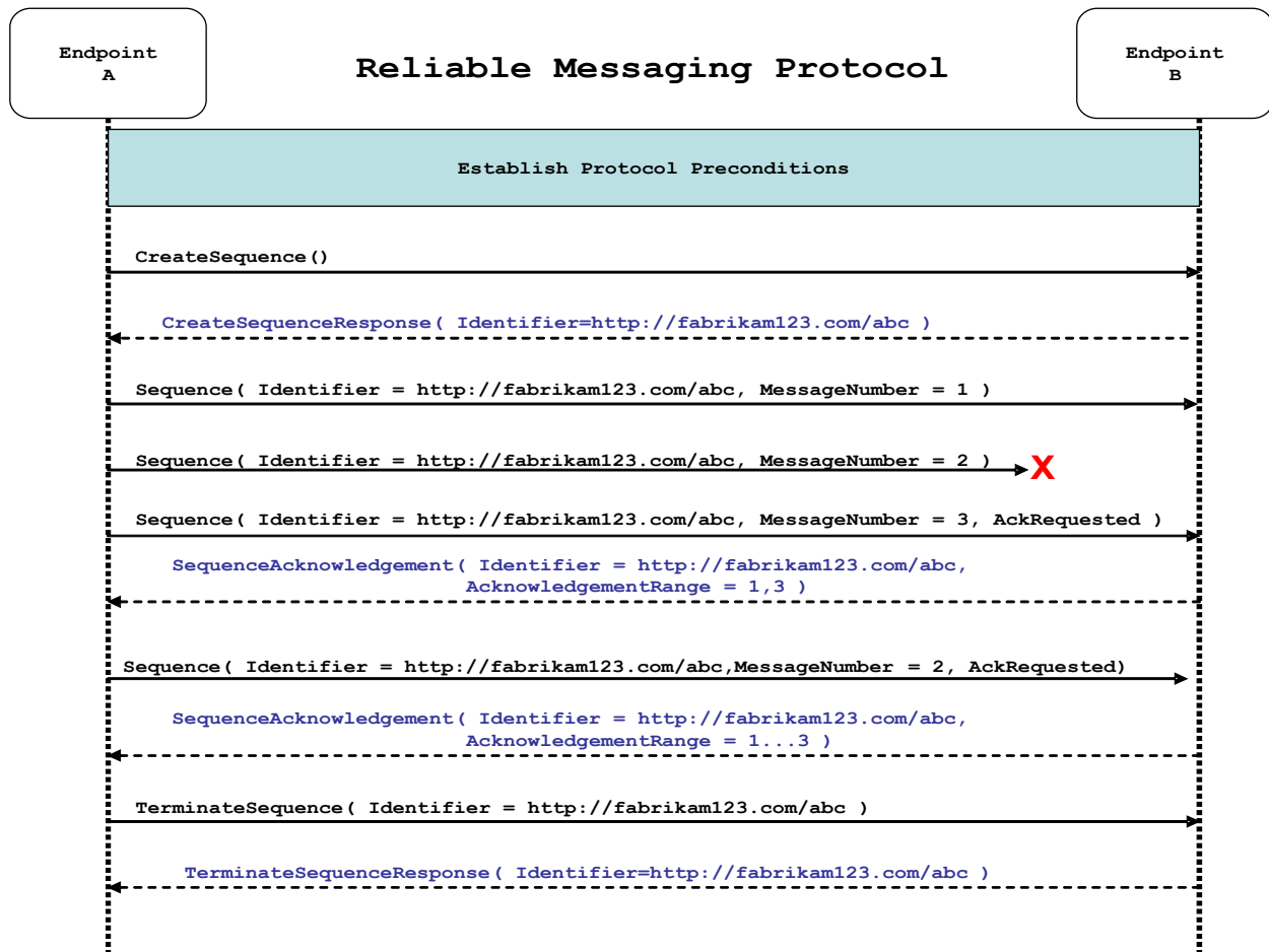
Figure 2: The WS-ReliableMessaging Protocol
