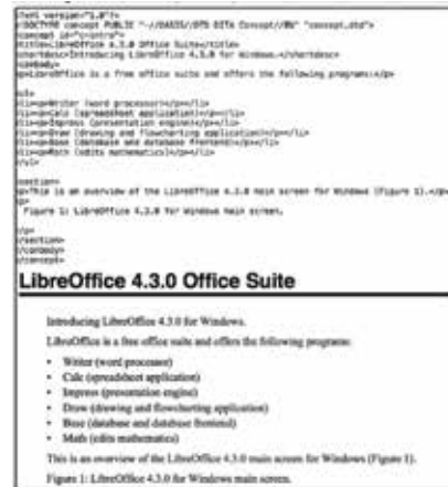
Figure 4: HDITA topic converted to DITA XML via Jotsom (top) and its PDF transformation (bottom) via the DITA Open Toolkit
