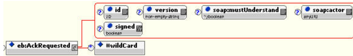
Figure 31 – Graphic representation of expanded view of the ebXML AckRequested element declaration
