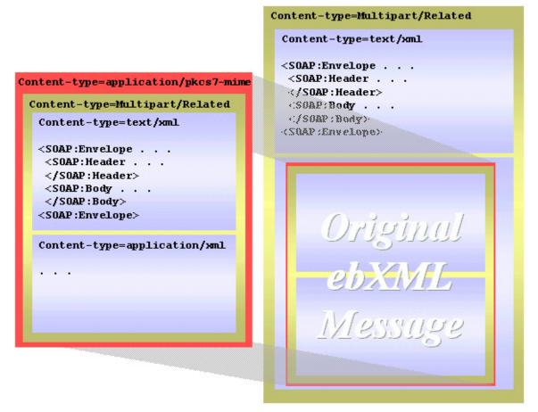
Figure 2 Encrypt before Encapsulate
