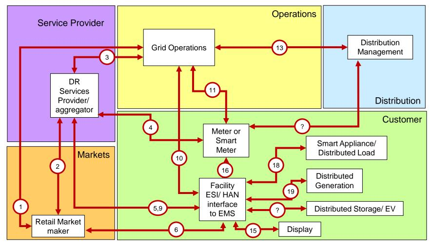
Removed Interfaces: 7 (meter doesn't get market signals), 8 (SP talks to devices through ESI), 12 (no grid op cnx to HAN device), 14 (not sure on this one), 17 (same as 18), 20-21 (meter doesn't talk to devices, but for AMI case ESI can be put in meter)
