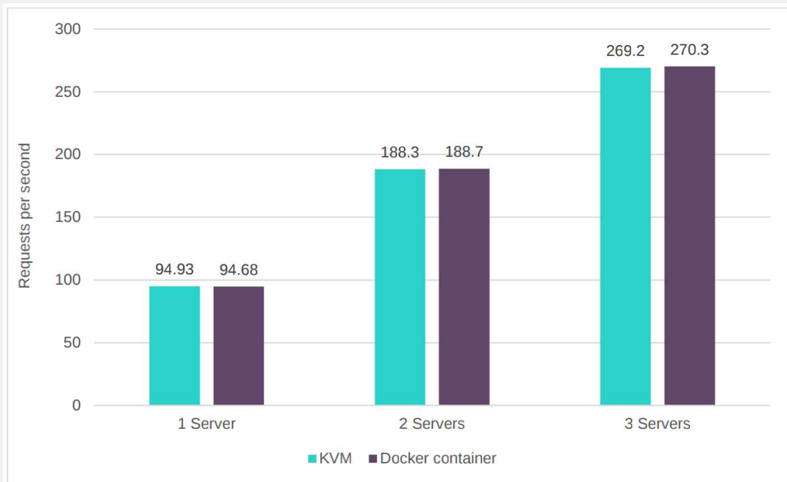
Figure 10. Comparison of Docker containers and KVMs (ProLiant DL580 Gen8 with RHEL 7.1)
